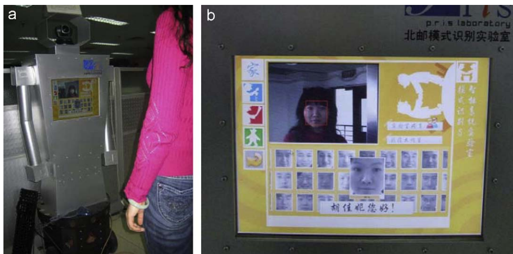
Fig. 14. The mobile robot recognizes the human face in the real-time video captured in the complex environment. The recognition is based on the single example stored in the gallery database as shown in (b). (a) Mobile robot. (b) Robot–human interface.
